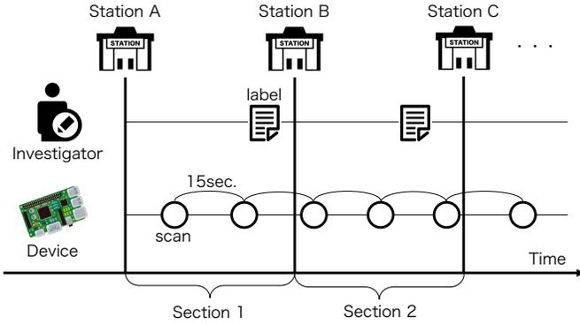
Fig. 2. Sensing process.
