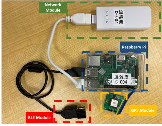
Fig. 1. System sensing device.
