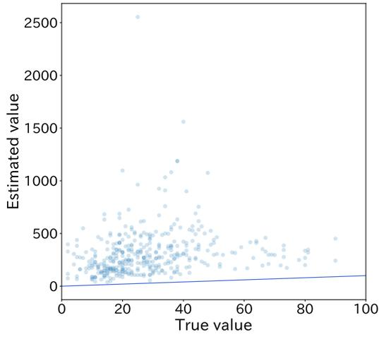
Fig. 5. Measured values (BD address counts) versus true values (passenger counts) obtained from raw data.
