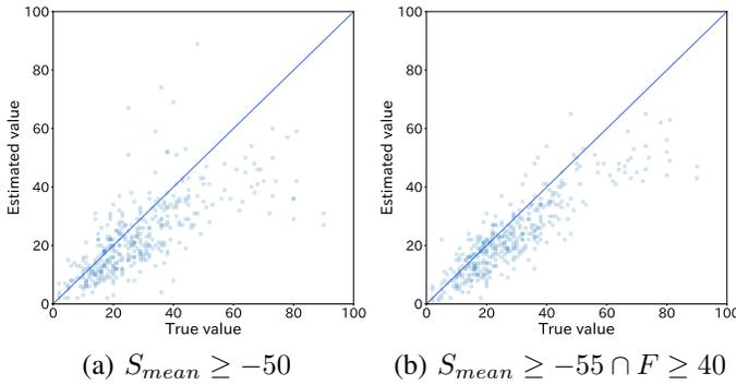
Fig. 6. Values estimated by LGBM (BD address count) versus true values (passenger count).
