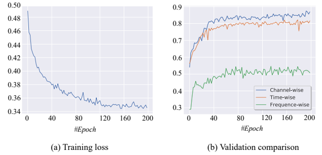
Fig. 2. (a) Training loss in channel-wise Transformer; (b) Accuracy in different ablation studies (time/frequency-wise Transformer comparing to ours)
